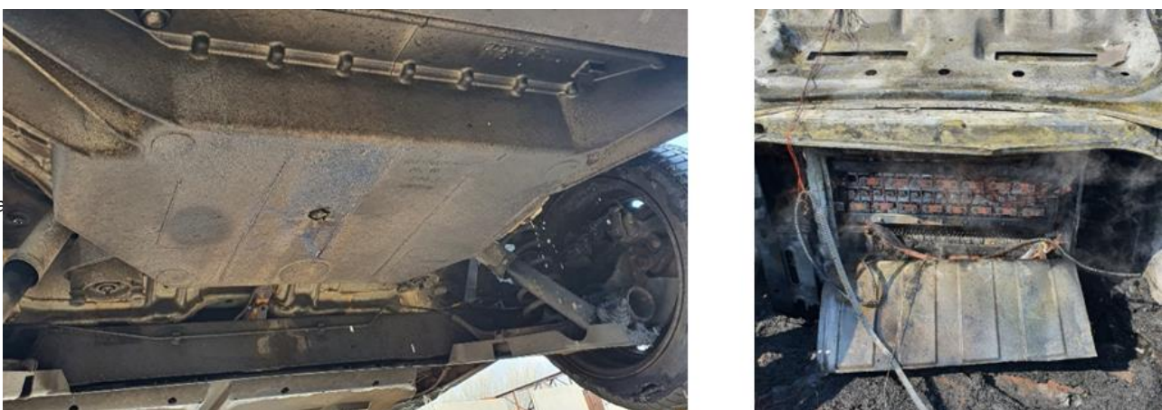
Figure 3.18: Post fire LIB pack of (a) pierced battery compartment and (b) the opened battery compartment after the experiment
