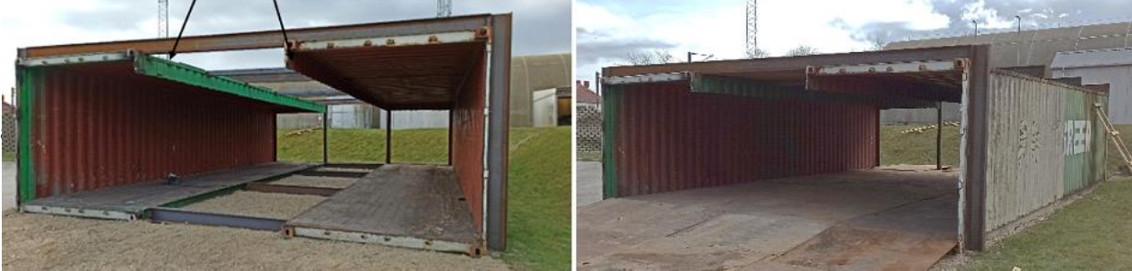
Figure 3.1: Experimental set-up (a) without the center ceiling and (b) with the center ceiling
