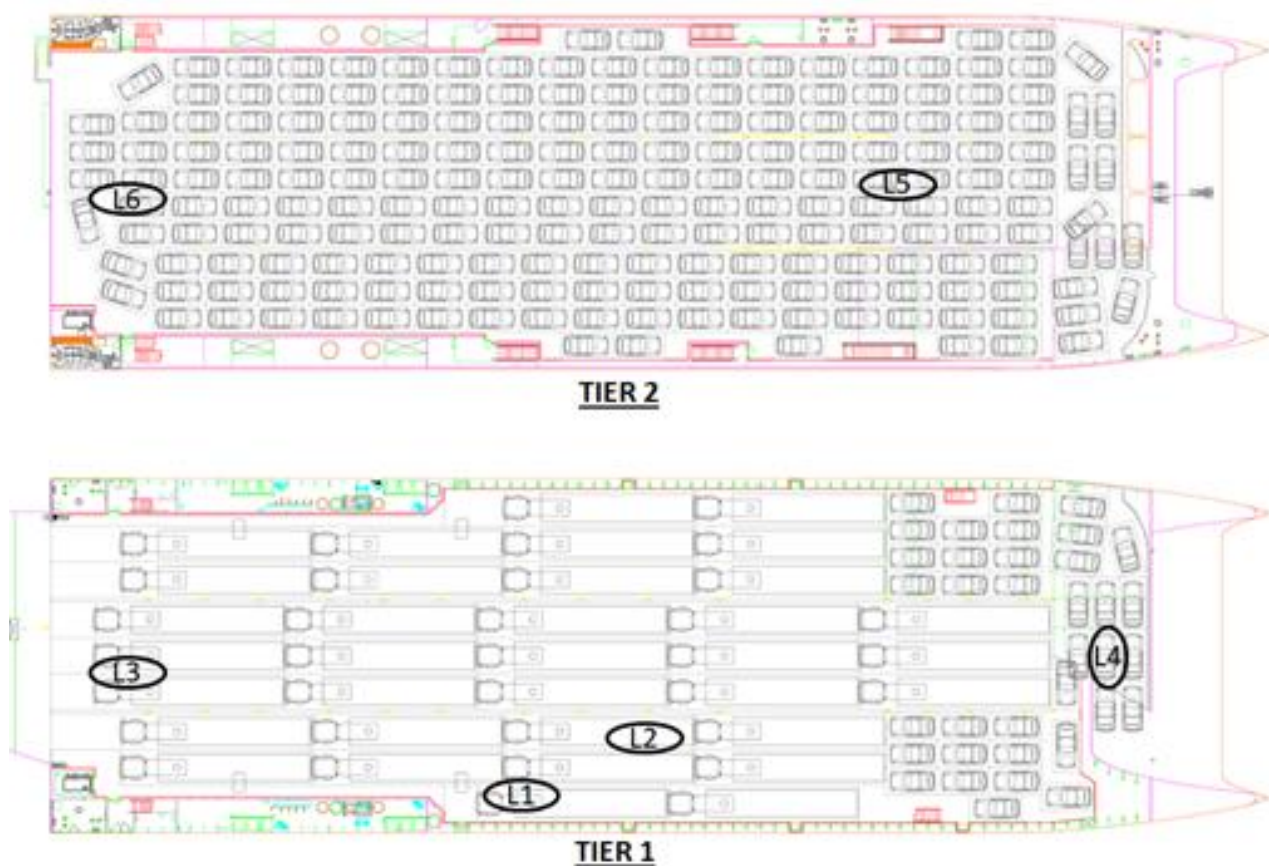
Figure 2.1: Locations of the vehicles ignited first in different fire scenarios on tier 1 and tier 2 of Molsslinjen EXPRESS 4
