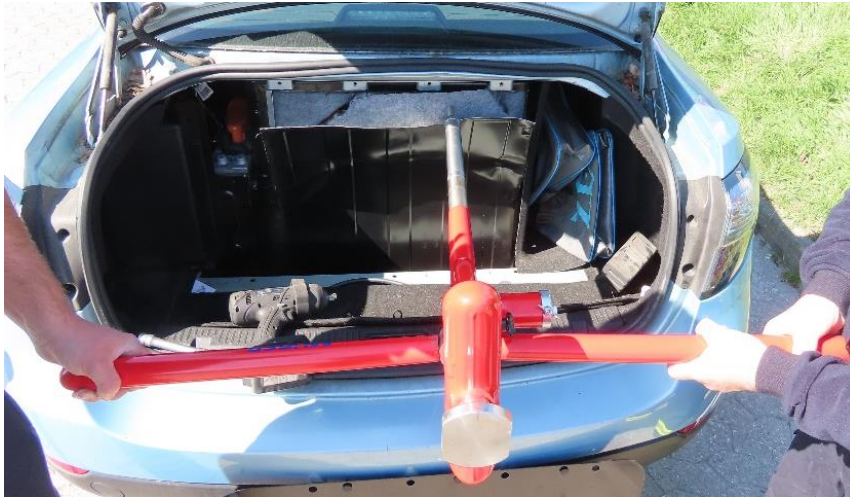
Figure 3.13: Holding the E-lance in place prior to striking
