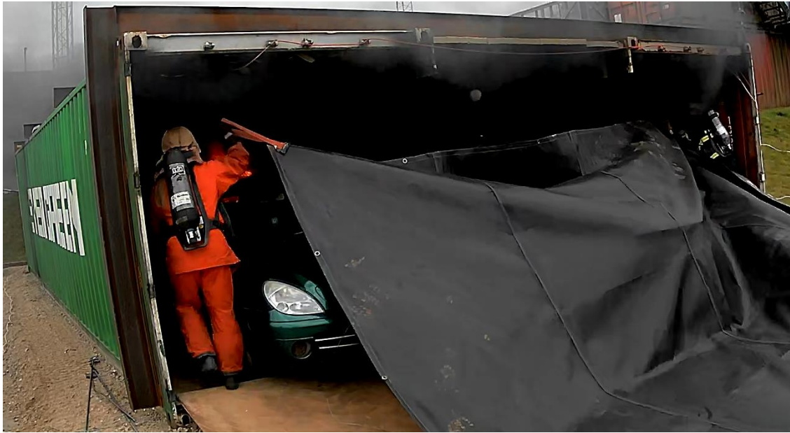
Figure 3.9: Bridgehill Car Fire Blanket being used during experiment 1
