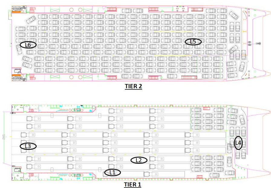
Figure 6.26: Locations of the vehicles ignited first in different fire scenarios on tier 1 and tier 2 of Molslinjen EXPRESS 4
