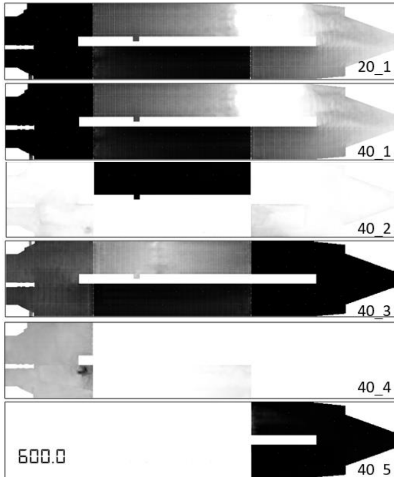
Figure 6.41: Smoke development seen from above at 600 s from the fire start in six different scenarios. Assuming the time of first detection activation is noted and its location is known, a fire in zone 1 would still be reachable 5 minutes after the fire starts, especially if a slow fire starts due to the failure of EV battery (see scenario 40_4).
